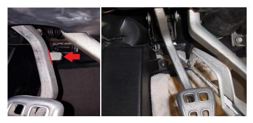
Step 2: Use a small hand file to smooth the pedal arm so the clutch stop assembly will mount flush on it.
