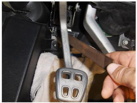
**Step 3:** Using a 5/32" allen wrench make sure the two outer set screws on the clutch stop are backed out and made flush with the inner part of the clutch pedal mounting area as shown below. This will prevent them from interfering with the mounting on the clutch arm, until you are ready to secure it using the same 5/32" set screws.
