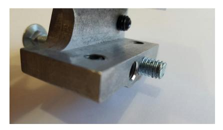
**Step 4:** Place the ECS clutch stop on the pedal arm in a location where the pedal tabs will touch both the clutch position sensor and bottom out on the small metal plate on the floor. Once it is located on the pedal arm secure the clutch stop in place by tightening the 5/32 set screws.
