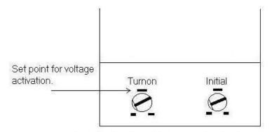
Turnon control will adjust from 1.7 volts DC to 4.9 volts DC. Full CCW is 1.7. Full CW is 4.9. Voltage can be adjusted by probing center terminal on Turnon control and adjusting to desired level.
