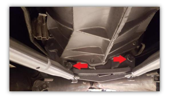
Strut bars assembly and install:
