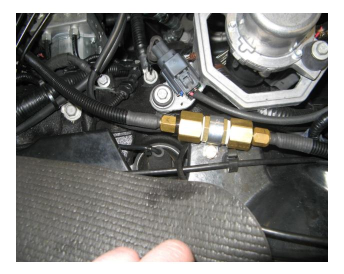
The nozzle goes installed in the charge pipe after the MAF sensor. Not before. \*Note this particular picture shows an IAT Breakout Kit added.
