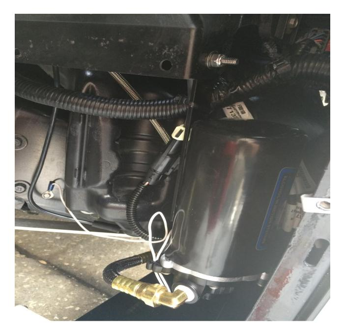
Next is attach the white wire to a chassis ground. A simple 5/16 self tapping screw to the plate handles this. Plug the pump harness into the pump. We are done with the inner fender portion of the install.
