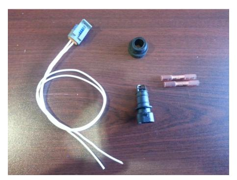
IAT Breakout: Both wires on the IAT sensor harness are reverse polarity. On the MAF sensor locate and cut the White/Light-Blue wire in pin #1 on the MAF sensor and the Black/Violet wire in pin #3 on the MAF and connect those to the wires from the IAT sensor harness using the supplied connectors.
