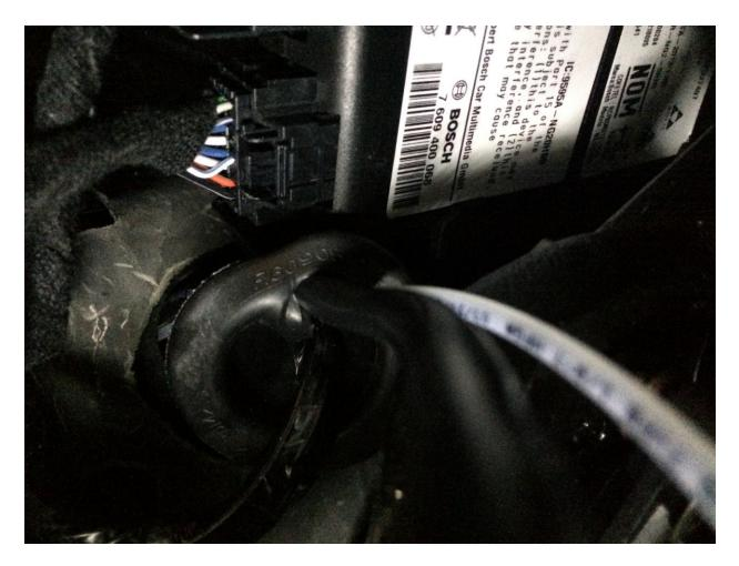
I used an Xacto knife and put a small slit into the rubber to run wires through it.
